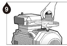
Install the Pulsarlube V unit on the lube point.
