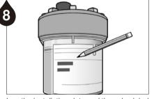
Log the installation date and the scheduled date of lube cycle completion on the label of the Pulsarlube V.
