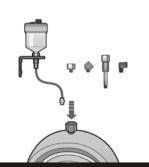
The Pulsarlube V is designed for single point lubrication only. Direct mount is always preferable. For applications not allowing any direct mounts, remotely mount the unit using appropriate accessories and keep the distance from the lube point as short as possible.
