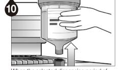
When the selected dispensing period of the Pulsarlube V has completed, remove the lubricator from the application.
