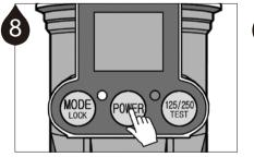
Press the POWER button for 2 seconds to turn the unit on.
