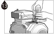
Install the Pulsarlube EX unit on the lube point. When the selected dispensing period has completed, replace the unit with the Service Pack according to step #3~7.
