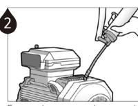
Ensure a clear passage using a manual grease gun. Note1 Remove any hardened grease by purging the lube point with a manual grease gun. Note2 The grease in the equipment and the grease contained in the unit should be the same or compatible.
