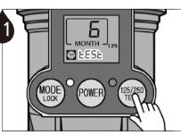
Press the TEST button for 2 seconds to run a test cycle and check for proper operation of the unit.
